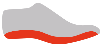
WIDE Wide lasts are wider along full-length, heel measure is wider than standard
